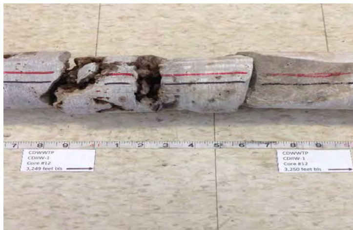
Figure 10. Core No. 12 (3,245.5 – 3,255.6 feet bls) showing fracture and dissolution features.
