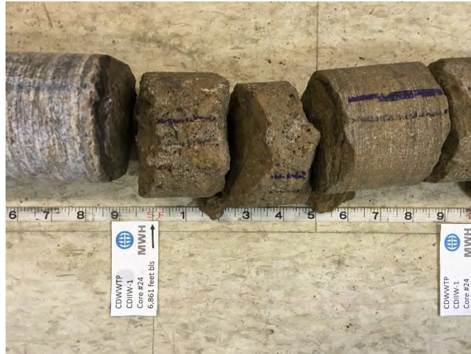
Figure 12. Core No. 24 (6,856 to 6,868 feet bls) obtained at CDIIW-1. This core might have cut through the base of the Pine Key Formation and into the top of the Corkscrew Swamp Formation, as seen in the change in lithology from top to bottom on the picture.
