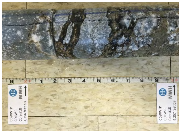
Figure 11. Core No. 18 (4,254 – 4,264 feet bls) showing Anhydrite, obtained at CDIW-1.
