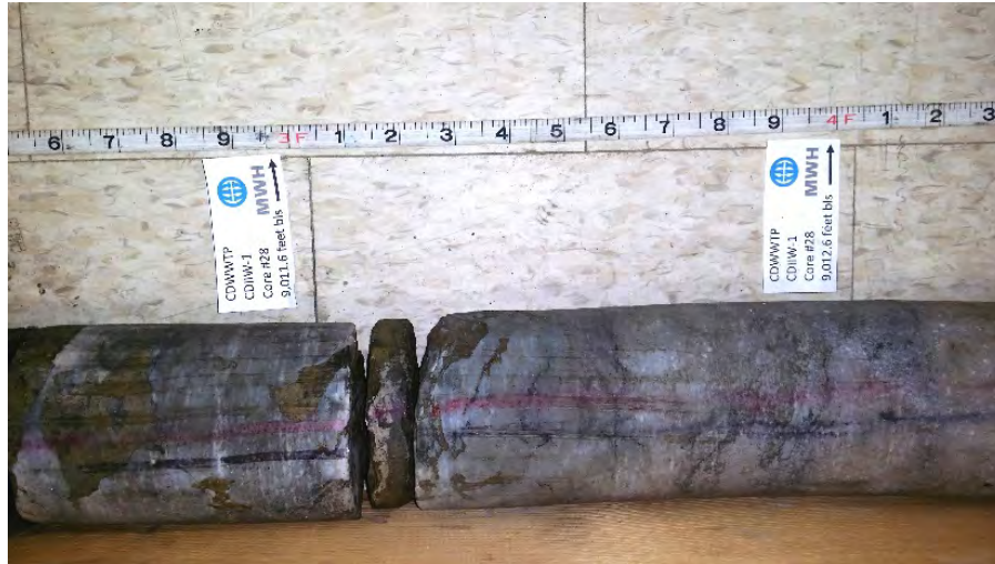
Figure 13. Core No. 28 (9,008.6 – 9,020.6 feet bls) obtained at CDIIW-1, showing some Anhydrite interbedded with limestone.
